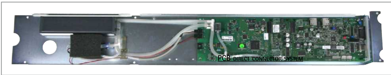
METAL SHEET CARRIER, ASSEMBLED (BPU, SMU, LIU)
